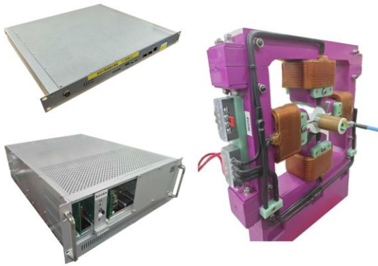
Figure 6: The DBPM processor, fast corrector power supply, and fast corrector magnet.
