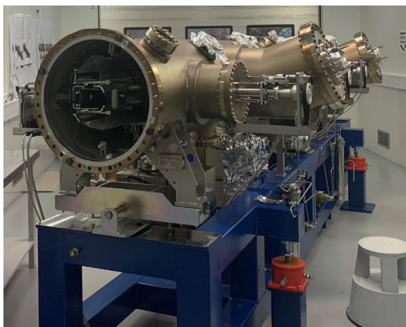
Figure 1: The SIS100 Extraction Septum currently build at DanFysik [1] in Denmark
