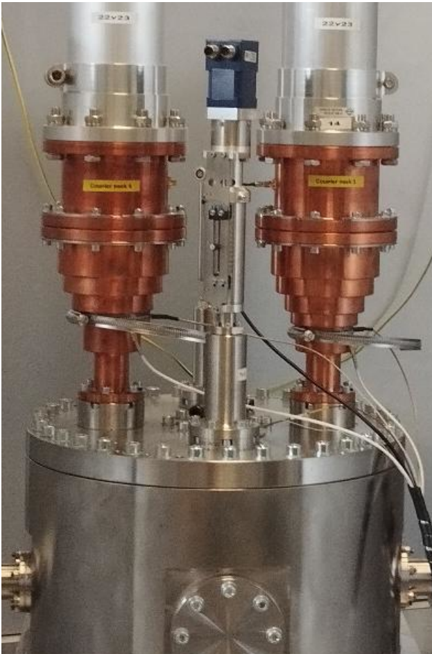
Figure 1: RFQ couplers attached to the testbox and to the coaxial waveguides.
