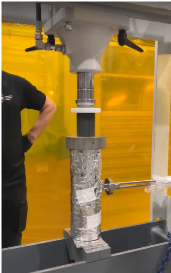
Figure 3: The pressing of the MBL IBS graphite core into the TZM enclosure. The core is a cylinder with h = 30 cm and r = 3.6 cm. Image courtesy of the ESS workshop.
