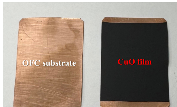
Figure 4: Photograph of the 2 \mu m CuO thin film and OFC substrate samples.
