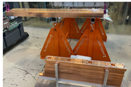
Figure 3: Assembly test for Helicoflex® seal.
