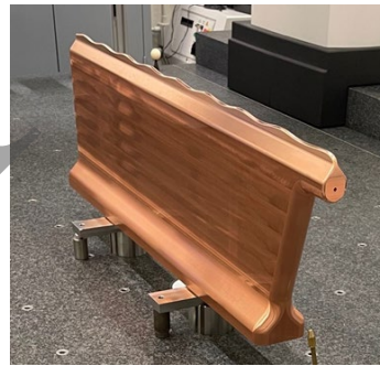
Figure 2: First vane of NEWGAIN RFQ.
