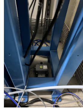
Figure 2: Beamline-floor measurement point with a Walesch MST-1031 tri-axial velocity sensor.
