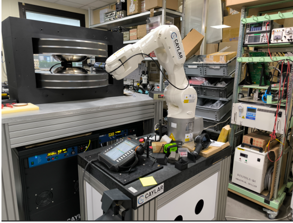
Figure 1: Magnetic field characterization system of the electromagnet, with a Hall probe mounted at the end of a six-axis robot.
