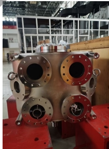
Figure 6: The fabricated 3 rd harmonic SC cavity is welded with a helium vessel.
