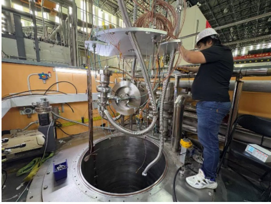
Figure 7: Two niobium cavities are put for vertical tests.
