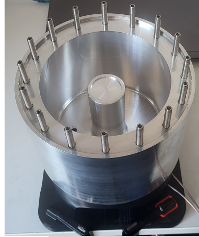
Figure 1: Final setup of the dedicated test cavity with removed top lid.
