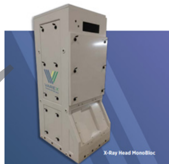
Figure 2: LINATRON “Tower” packaging with Solid State Modulator (SSM) used on a 6 MeV Mi6SSM (diode e-gun), but now the similar packaging is used for Mi6SSM-T (triode e-gun), both are subsystems for security screening systems.
