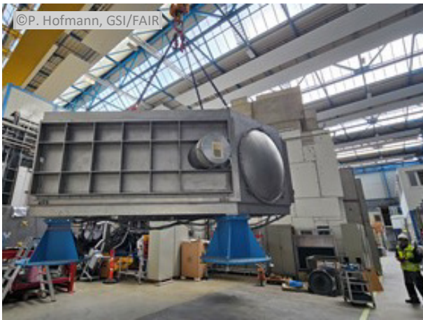
Figure 10: Lifting test of the GLAD vacuum chamber.
