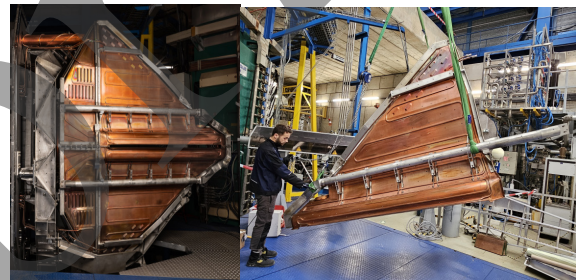
Figure 5: HF cavity and cooled outer casings of a CSS cyclotron.
