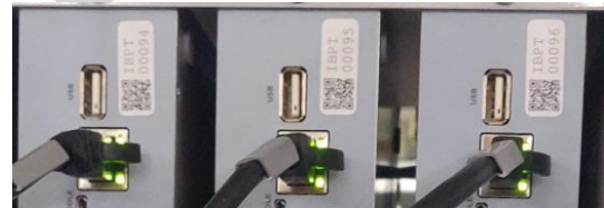
Figure 2: Basic labels. This minimal label is used during the initial registering of new devices based on an already existing generic entries in the database.
