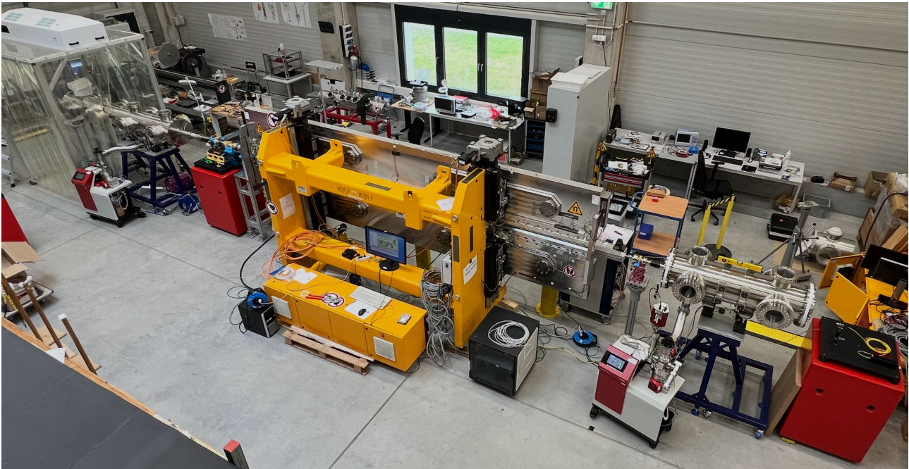
Figure 1: SUNDAE2 measurement setup with a 5 m long U40 permanent magnet undulator. The entire setup spans 11.2 m. From left to right: DN350 vacuum chamber hosting a xyz adjustment for the thin wire and the drive system and parking area for the Hall probe sledge. On the red concrete stone follow the laser based detections systems for the pulsed wire. The large chamber on the right of the undulator hosts the tension system for the Hall probe sledge and xy stages for the wire. On the red stone on the right the interferometer for distance control of the Hall probes is placed. Large windows allow visual control and large DN250 doors allow quick access for installing the wire. Due to the limited conductance of the electron beam chamber, two pump carts equipped with scroll and turbo pumps provide the vacuum. Optionally ion getter pumps below the large chambers enable vibration-free vacuum.
