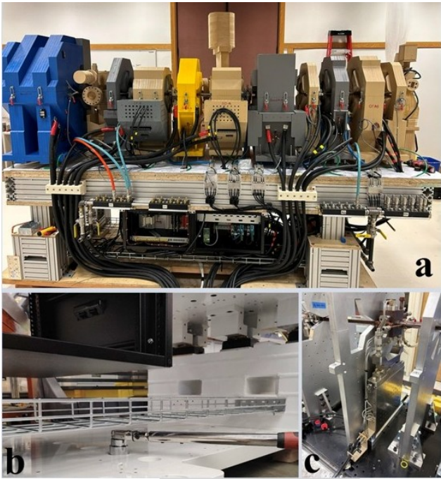
Figure 6: SR Module Mockups for interface verification: (a) mockup, (b) electrical cable tray integration, (c) vacuum chamber test fits.
