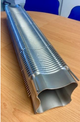
Figure 3: Wire eroded model thin-wall quadrupole chamber (star-shaped) with LHe cooling pipes.
