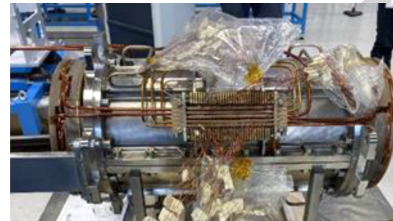
Figure 2: Multipole corrector magnet manufactured in industry.
