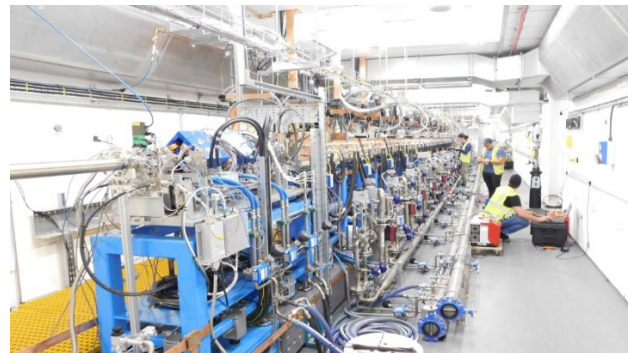
Figure 5: AVO Linac test facility at Daresbury Lab during commissioning : ECR source (from DREEBIT; 2,45 GHz), RFQ (Design by CERN, end Energy 5 MeV), SCDTL cavities (Design ENEA, Italy; end energy 37,5 MeV) und CCL cavities (up to 230 MeV).
