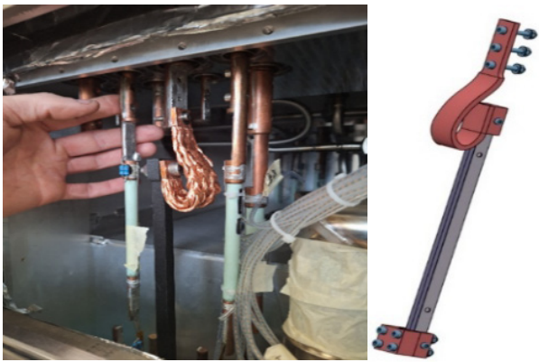
Figure 14: New design of HTS current lead.
