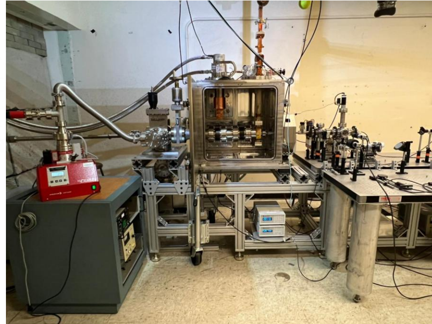
Assembled load lock behind cryostat
