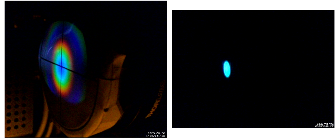
Undulator radiation on screen FS with wide and narrow iris
