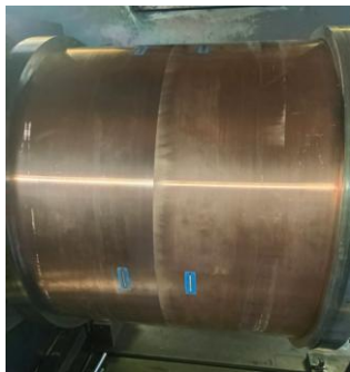
3m-long absorber in electron beam welding
