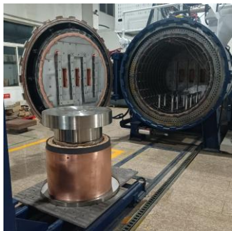
Single-block absorber in brazing
