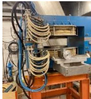
Test stand for RF material qualification using magnetic fields up to 1.2 T and pulsed voltages
