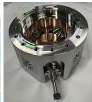
Test stand for RF material qualification using magnetic fields up to 1.2 T and pulsed voltages
