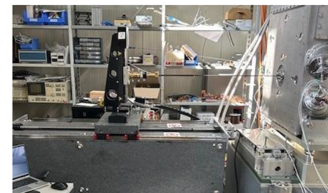
Magnetic measurement system 3D hall probe
