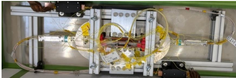
Double Racetrack of HTS (ReBCO) insulated (soldered) tape-stack cable tested at PSI
