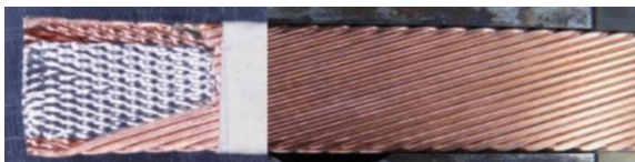
Rutherford cable (21 high-current-density strands)
