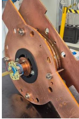
5x 12 mm wide Non insulated HTS coils
