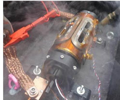
Sextupoles made of 6 racetrack HTS coils (coated HTS tapes at PSI)
