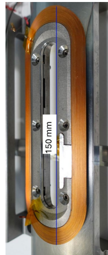
Sextupoles made of 6 racetrack HTS coils (coated HTS tapes at PSI)
