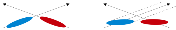
Figure 9: Bunches colliding with a crossing angle without crab crossing (left); with the crab crossing (right).
