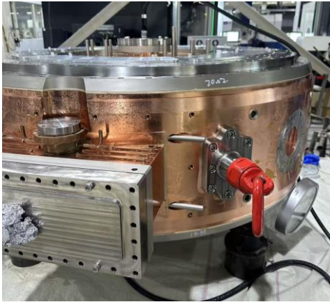
Figure 7: A prototype of the room-temperature TM020 RF cavities for the collider rings.
