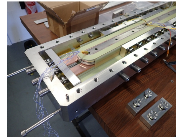
NARSIL stack in the structure Narsil MI coil [T. Lecrevisse et al.]
