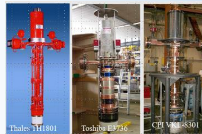
Frequency: 1.3 GHz Peak RF power: 10 MW Efficiency: 65%
