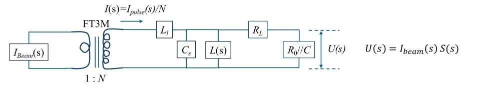
In case of the signal calibration using 1 turn coil and single rectangle pulse signal, output voltage can be expressed as,
