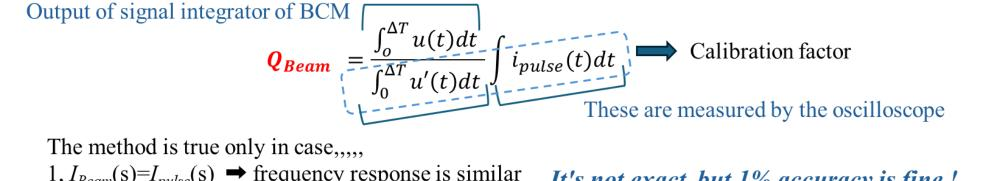
1,  $I_{Beam}(s) = I_{pulse}(s) \implies$  frequency response is similar It's not exact, but 1% accuracy is fine ! 2, Transmission efficiency is unity  $\Rightarrow \chi(s) = 1$
