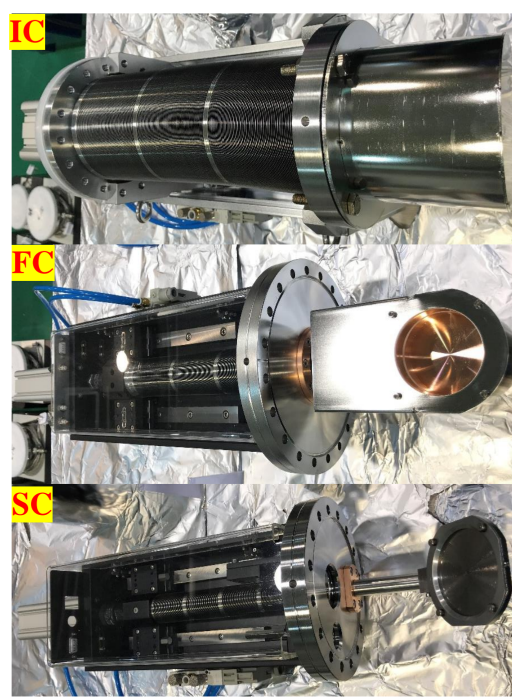
Fig. 3 Prototypes of the SC, FC and thick IC. All the detectors are driven by pneumatic device
