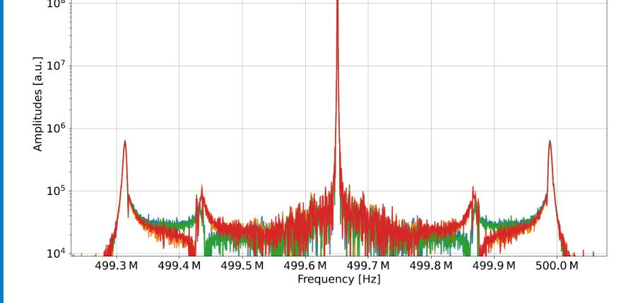
Tune sidebands are clearly visible during injection with stored beam at nominal current: horizontal tune is at 0.347 kHz from the carrier, while vertical tune is at 0.231 kHz (respectively 0.4 and 0.2 of the revolution frequency).
