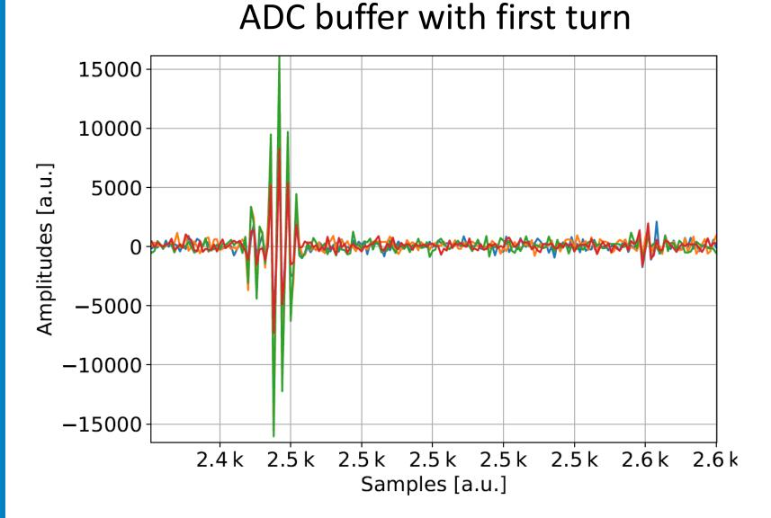
After extracting a single bunch of 0.75 mA coming from the booster, we inserted a fluorescent screen in the storage ring to stop it after one turn. The residual charge that is not completely stopped by the screen can be seen exactly 130 samples after the main signal, corresponding to one turn.
