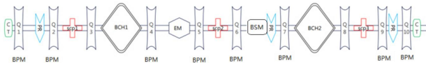
10quads, 2 bunchers, 3.04 meters long
