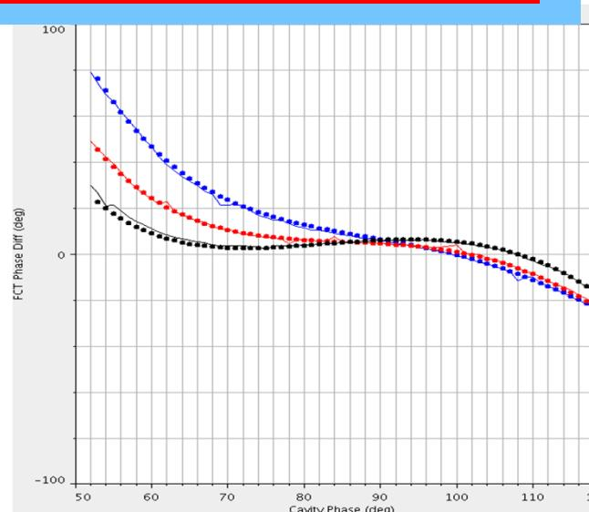
Beam energy measured with two methods
