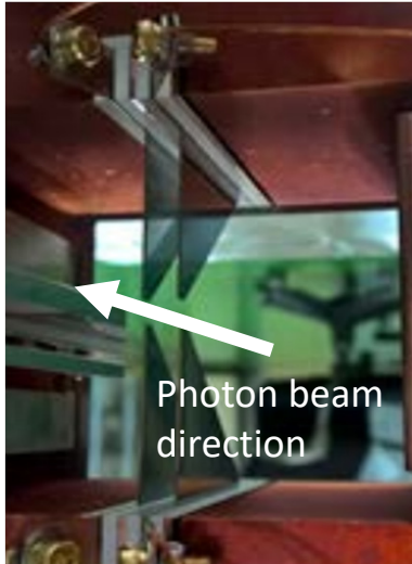
Initial version of PBPM with tungsten blades
