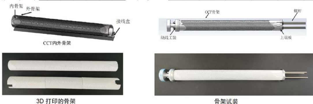
QD0 former drawing and 3D printing dummy former
