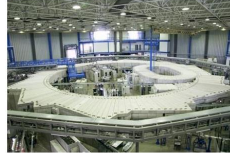
LNLS (1997) 1.37 GeV \epsilon_x = 100 \text{ nm} , \epsilon_y \sim 1 \text{ nm} , I = 250 \text{ mA}
