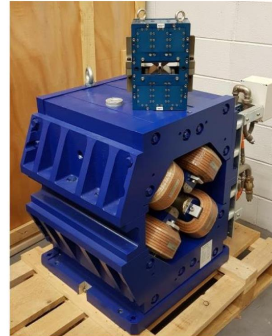
Upgrade Permanent magnet quadrupole prototype (top) Present Electromagnet quadrupole (bottom)
