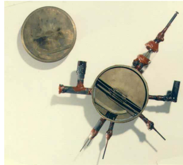
First 4-inch cyclotron, 80keV protons A number of cyclotrons of increasing size followed.
