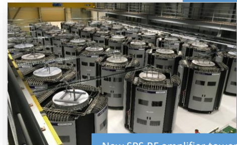
New SPS RF amplifier towers
