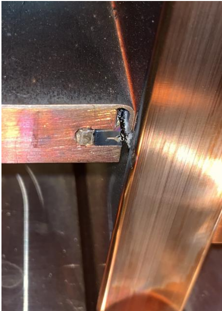
Damage on the stem tuning plate interface
