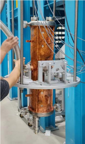
HWR010 Cu/Nb cavity mounted on vertical test stand
