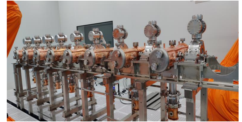
The assembled 9 HWR010 Cu/Nb cavities string
