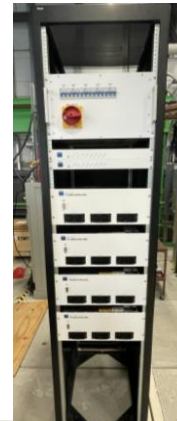
644 MHz 20 kW amplifier installed at SRF bunker
