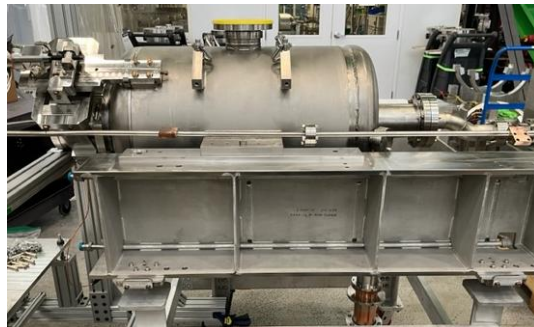
S65 Test Cryomodule: Cavity, FPC, tuner, rail, hood
