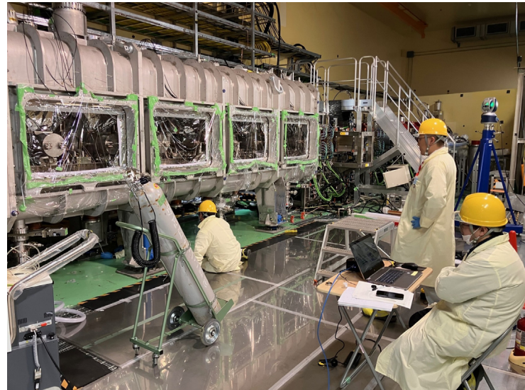
Final alignment of the cryostat
