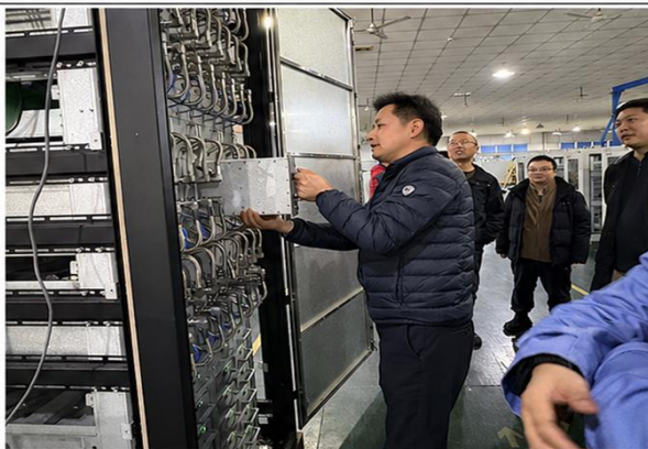
(c) Hot-Swapping of a Faulty PA Module During Operation
