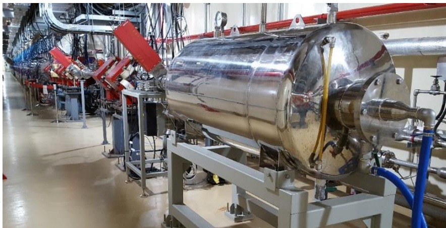
Beam dump (neutron generation target)
