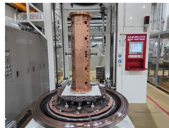
In-house section brazing setup
