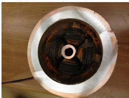
Cutting view of the drift tube Poor insulation between windings and yoke
