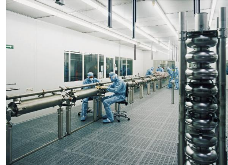
TESLA cavity = 9-cell superconducting Niobium cavity Booster cavity = one TESLA Cavity in a cryostat, Accelerator Module = 8 TESLA Cavities in a cryostat
