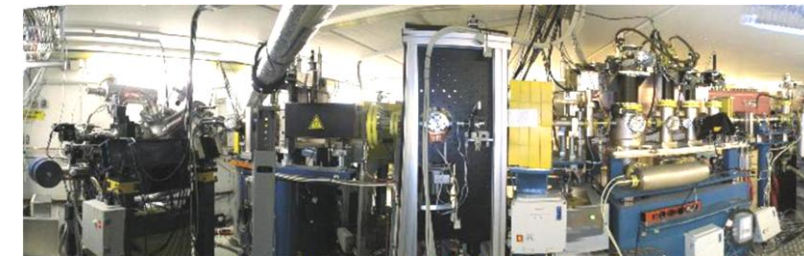
TESLA cavity = 9-cell superconducting Niobium cavity Booster cavity = one TESLA Cavity in a cryostat, Accelerator Module = 8 TESLA Cavities in a cryostat
