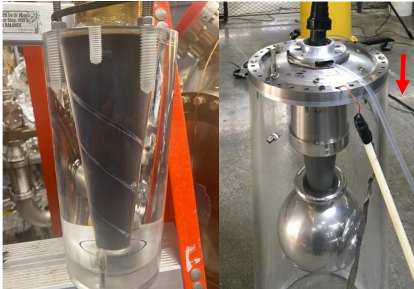
Custom-designed HV plug with cooling channel
