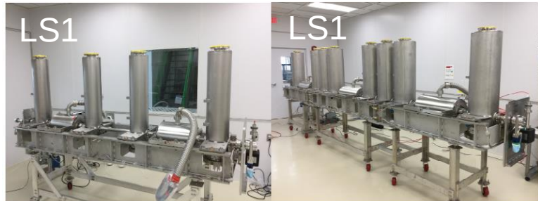
4 \beta = 0.041 : 4 QWRs x 2 Solenoids 11 \beta = 0.085 : 8 QWRs x 3 Solenoids
