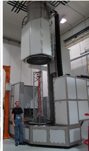
Vacuum brazing furnace at PSI
