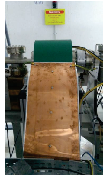
Copper sheets installed on one of pulse elements and another one to DCCT+FCT shield
