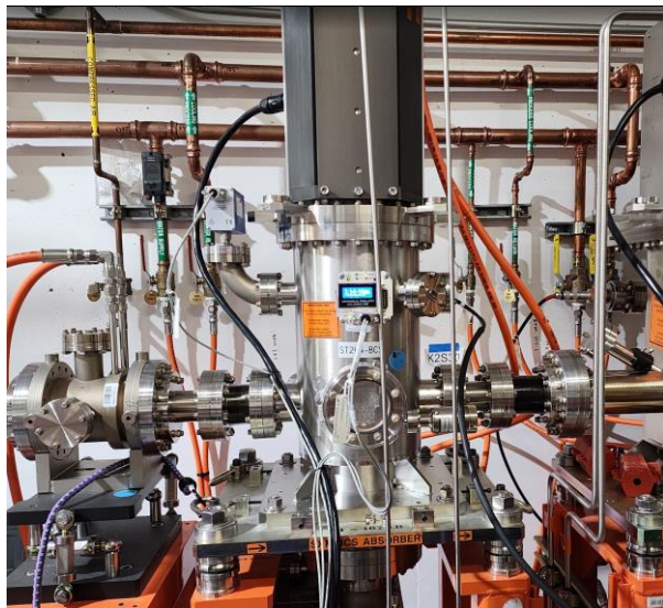
Soft X-ray beam test stopper in LCLS Front End Enclosure (FEE) / located just prior to the photon experimental hutches (near hall) / SIM electronics located ~150 feet away
